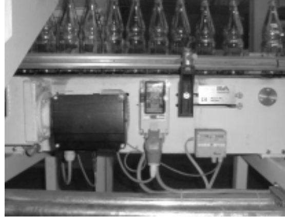
Figure 5. AS-i slave in combination with a frequency inverter motor
