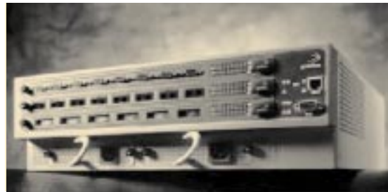
Figure 9. Storage Area Network (SAN) Switch.
