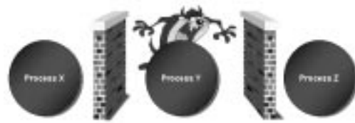
Figure 2. MMU erects "walls" around code and data and tames errant processes.
